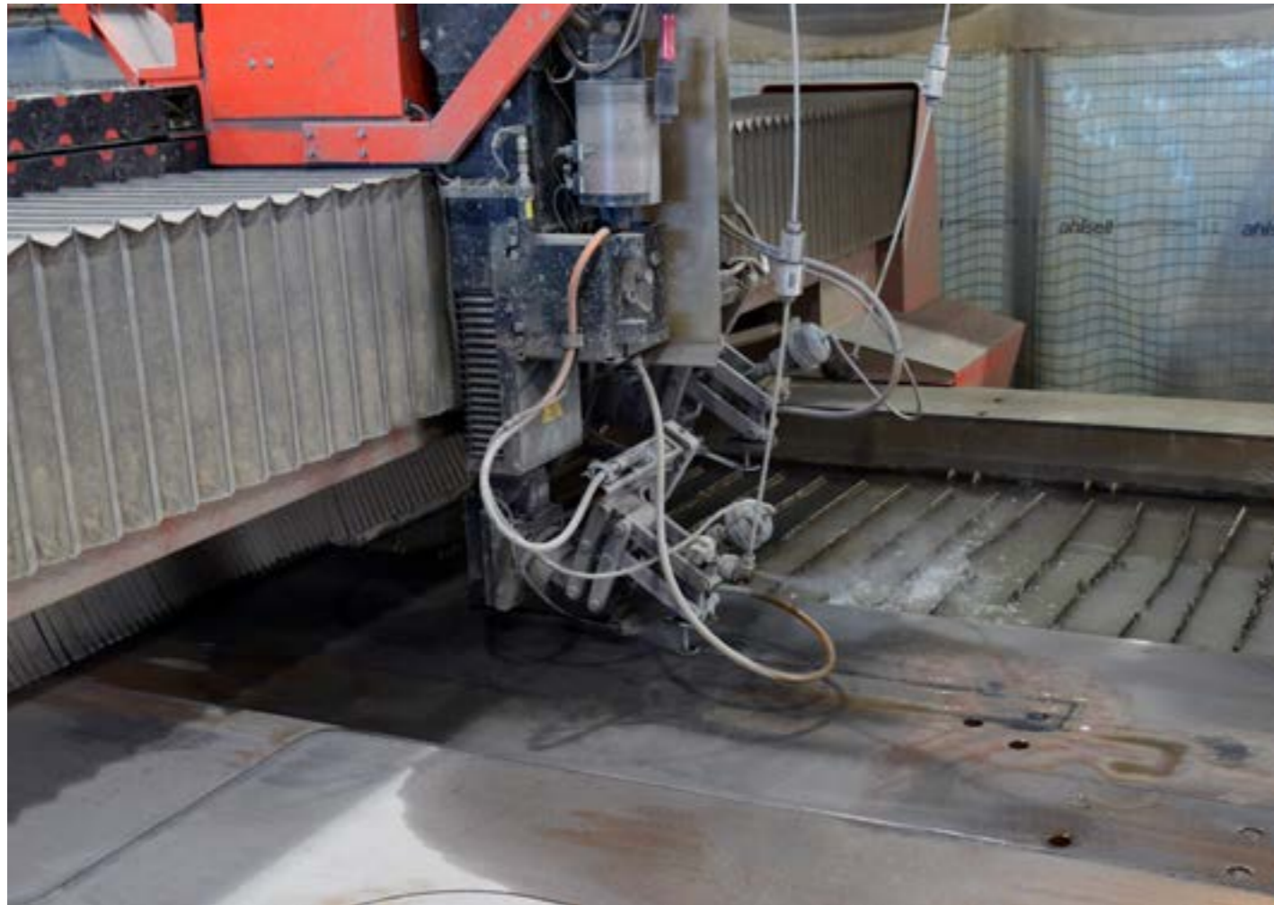
LKAB Mekaniska's 5-axis waterjet cutting machine.
